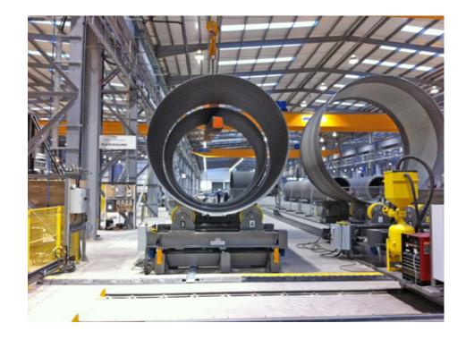
The fit-up system is engineered with movable wheels to manipulate each can, ensuring plate offset adjustments for seamless integration around the entire circumference during tack welding. Customisable with a range of add-ons, including conventional rotators, SAR rotators, additional wheels for precise can positioning, and options for hydraulic or electrical movement of the rotators, the fit-up system is adaptable to various setups.
